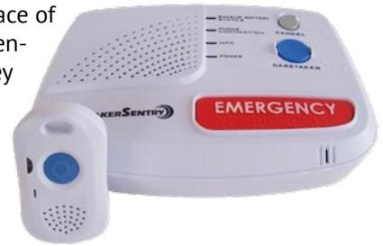
The base unit is connected to an existing landline telephone and is able to dial through to Central Station. Dispatchers can communicate with the customer and send help. Depending on the situation, dispatchers can send friends or family to check on the customer or notify police, fire or ambulance services if it is an emergency. With the two way communication pendant, the customer can communicate with Central Station outside of the home, up to 600 feet away.
